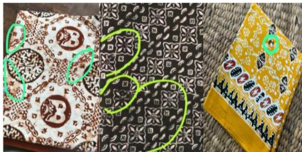
Figure 1. Types of Uneven Color Defects, Broken Wax Defects, Color Out of Motif
