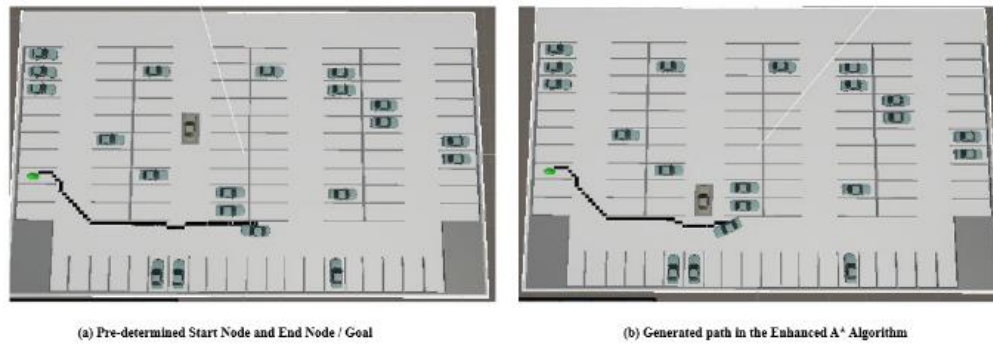
Figure 4: Performance of the Traditional and Enhanced A* Algorithm Under Various Conditions (Moving Objects)
